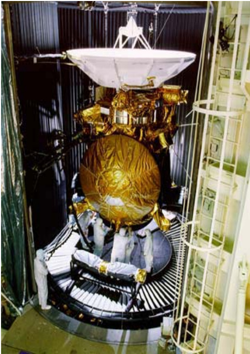
Figure 1: Integration of the Cassini / Huygens spacecraft; the persons at the basement provide a reference for size.
